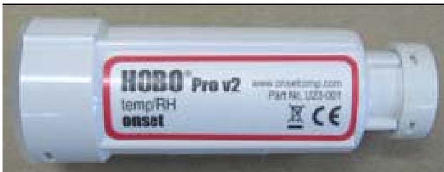
Picture III.1: Data logger with integrated temperature and humidity sensor
