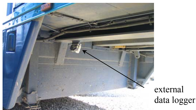
Picture III.3: Example of a data logger, installed under a semi-trailer for recording external temperatures/humidity
